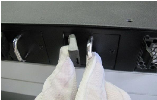
Figure 2-4 Removing the Filler Panel from the Power Module
