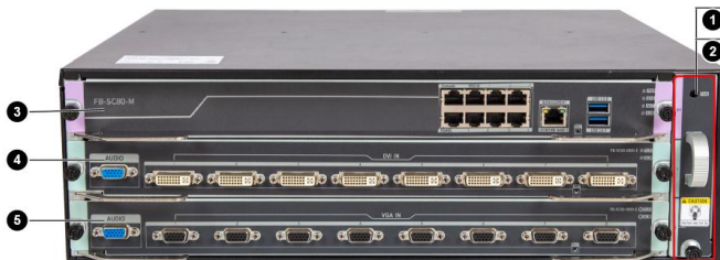
Figure 1-1 Front View of a 4-Slot Device
