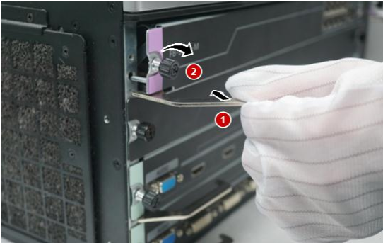
Figure 2-3 Fixing the Control Board and Service Boards
