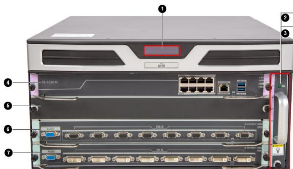
Figure 1-2 Front View of a 6-Slot Device
