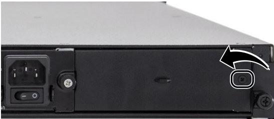
Figure 2-6 Removing the Filler Panel from the Power Module
