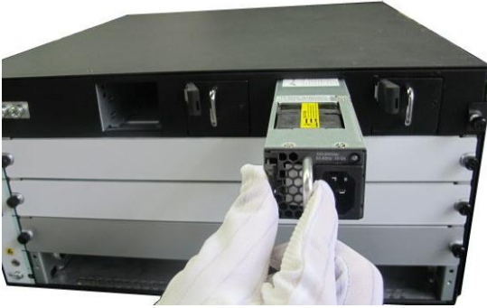
Figure 2-5 Installing the Power Module
